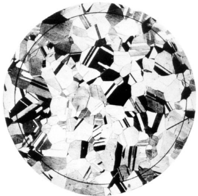
FIG. 3 Example of Twin Grains (Contrast Etch) from Plate III. Grain Size 0.090 mm at 75X
